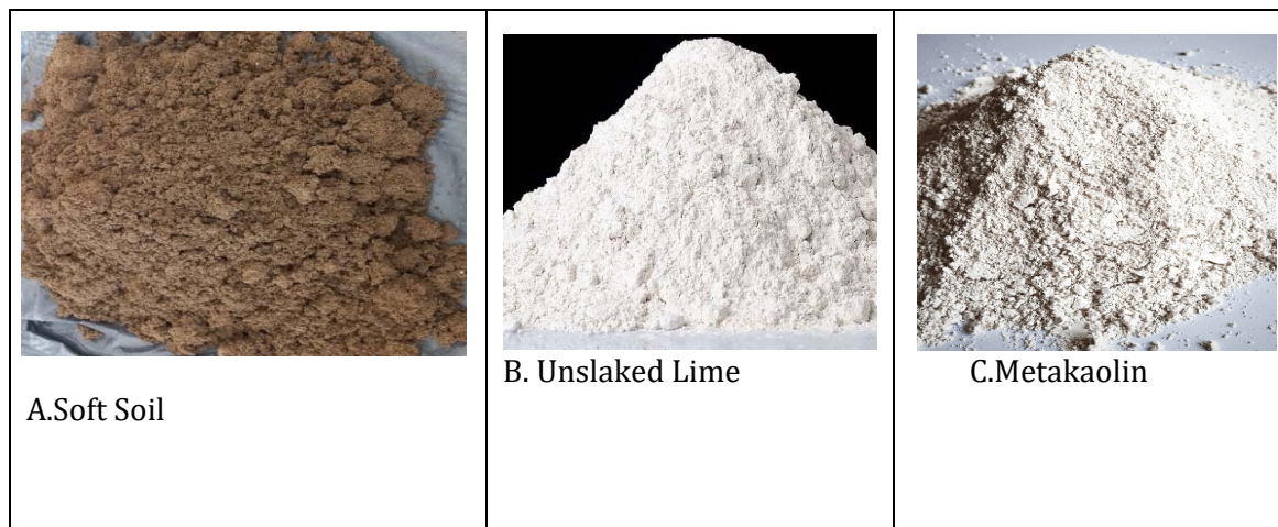
Figure 1. Soft Soil, Unslaked Lime, and Metakaolin
